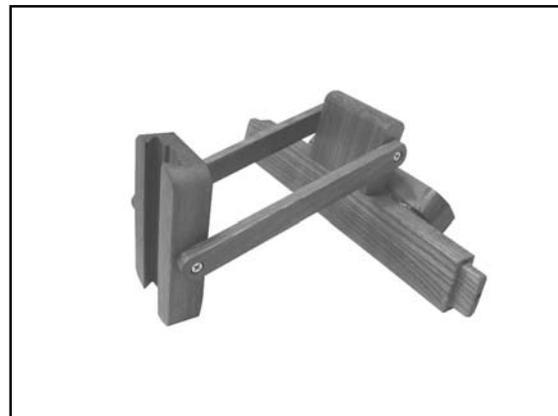
*STEP 1: Using the screws from bag A fix the top support bar of the A-frame to the mast guide exactly as shown. NOTE: In Step 2 ensure that the piece with the metal strip is placed into the A-frame support and not into the shorter back leg support.*
