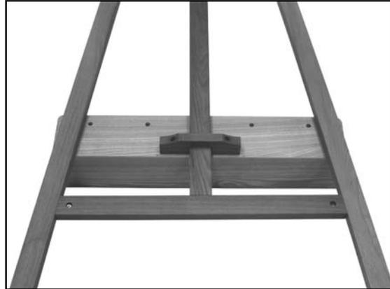
*STEP 10: Fix small "C" shaped piece of wood over central A-frame column onto accessories tray with screws from Bag F as shown.*
